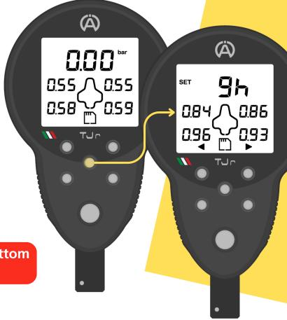
To select the desired SET, use the upper right and left buttons. Once you have reached the desired SET, press and hold the action button
