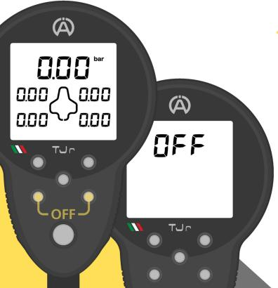
To turn off the TJr, briefly press the two lower buttons simultaneously on any page
