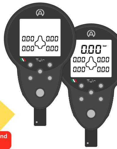
To assign a pressure to a wheel, when the pressure is displayed in real time at the top of the screen, press the corresponding button on the TJr
