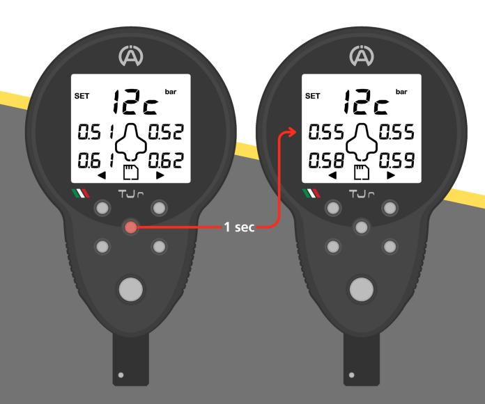
To scroll through the SETs quickly, hold down one of the side buttons
