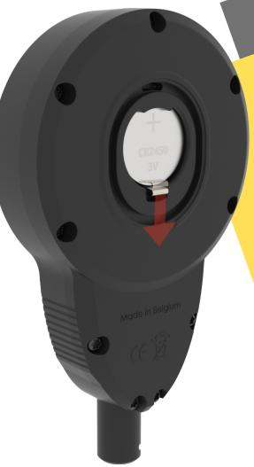
Insert the new battery with the positive end facing upwards and push it into the TJr until the latch clicks into place
