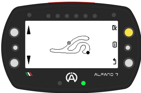
The lower right LED will turn green to indicate that the line is far enough from the existing lines on the track
