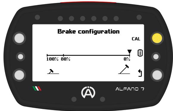
When the position corresponding to 0% is confirmed, the calibration is completed and the real-time status of the brake pedal is displayed again
