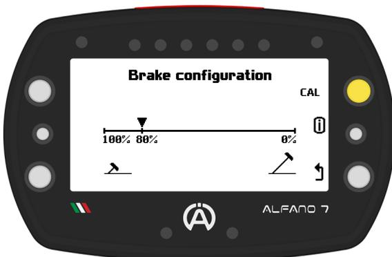
The value corresponding to the pedal being fully depressed is 80% to monitor the wear of the brake pads
