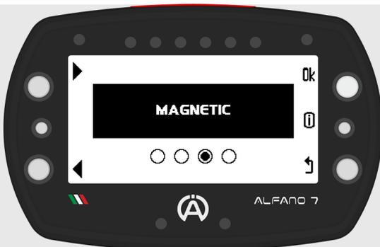
The classic magnetic mode allows only the use of the magnetic/IR sensor
