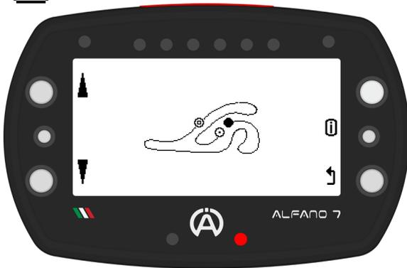
The LED lights up red if the inserted line is too close to a line already present on the track
