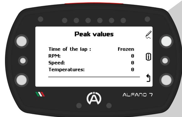
If a **freezing time** is set, when a **maximum/minimum value** is reached on this channel, Alfabo 7 will **block the relevant widget** (if present on the race screen used) for the **set time**. If, during the **freezing time**, the **maximum/minimum value** shown on the display is **exceeded**, the **value is updated** and **remains frozen** for the **set time**.
