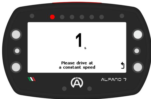
While learning the gear, the gear that the device is configuring is indicated in the center of the screen
