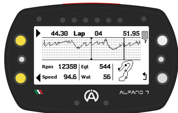
The graph at the centre of the screen displays the engine RPM throughout the lap
