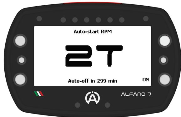
From factory settings, the device will enter **standby mode** after **15 minutes** of **inactivity**
