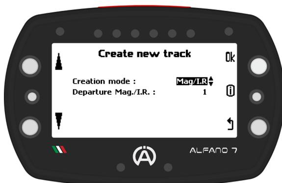
Confirming the "Create new track" item with the "ok" button will open the configuration menu for creating the new circuit if the instrument is receiving the GPS signal
