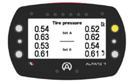
Press the top right button to display the tire's internal air temperatures
