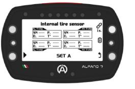
The Alfano 7 can be connected to 8 A1210 sensors: 4 in SET A and 4 in SET B
