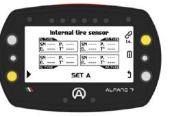
The Alfano 7 is able to automatically recognise the SET of the sensors mounted on the vehicle wheels, even during a tire change in the pit lane
